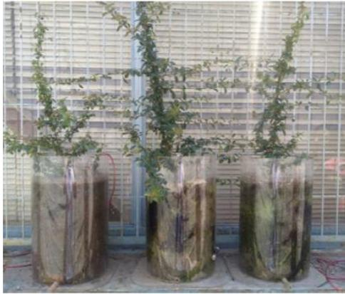
Fig. 1: Use of *Stenocarpus sinuatus*-based reactors in Plant Microbial Fuel Cells.
